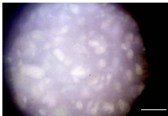
Fig. 2 Optical microscopic picture of colloidal particles of green tea. Objective lens \times 40 , eye lens \times 10 , length of the bar 25 \mu\text{m}
